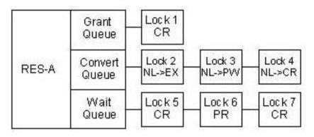
If you release Lock 1, the lock manager can grant Lock 2, the EX lock waiting at the head of the conversion queue. Because the mode requested by Lock 3 is not compatible with an EX mode lock, no other request on the convert queue can be granted. The following figure illustrates the lock resource's queues after the lock conversion operation.
