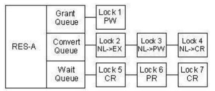
If you request a down-conversion of Lock 1 from PW to CR, the lock manager can grant the conversion request because a CR lock is compatible with the mode of the most restrictive currently granted lock. (Lock 1 itself is the most restrictive currently granted lock; a lock cannot block itself.) Note that the lock manager performs an in-place conversion of Lock 1, without adding it to the end of the convert queue.
