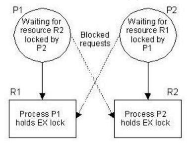
The processes in this example are deadlocked. Each process is blocking the other and neither is able to do any work. To break this deadlock, the lock manager cancels one of the blocked requests and notifies the requesting client by returning a deadlock status.
