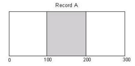
The lock manager does not maintain distinct lock objects. Rather, it keeps a database of which regions of the resource are locked. The lock manager does not keep locks separate. Instead, it coalesces overlapping locks of the same mode. If an application has an exclusive lock on a region from 0 to 10 and then obtains another exclusive lock on the region from 11 to 20, do not assume that two locks exist. Rather, consider the region from 0 to 20 locked.
