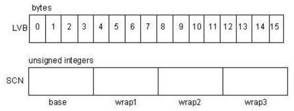
You define the range of the SCN counter by specifying, in the bit\_len parameter passed to the dlm\_scnop routine, how many bits are used to represent its value. The value of the bit\_len parameter controls which bits in the four fields are used.
