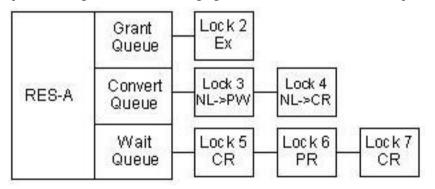
If you request a down-conversion of Lock 2 from EX to NL, the lock manager grants the conversion in-place because a NL lock is compatible with the mode of the most restrictive currently granted lock (EX). The lock manager checks the convert queue to see if the change allows any blocked conversion requests to be granted. The lock manager can grant Lock 3 and Lock 4 on the convert queue because PW and CR are compatible.
