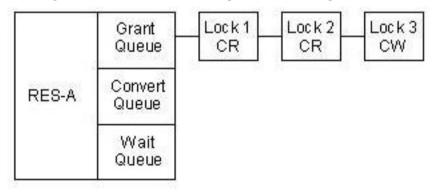
A lock conversion request that cannot be granted transitions into a converting state. The lock manager moves locks that are in converting state from the grant queue to the end of the convert queue. Locks that are in the converting state retain the lock mode they held in the grant queue.
