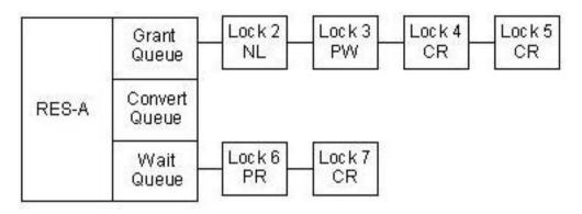
If you release Lock 4 and Lock 5, the lock manager cannot unblock the locks on the wait queue because the mode of Lock 6 is still not compatible with the most restrictive currently granted lock.
