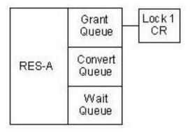
If the lock manager receives another request for a lock on RES-A at mode CR, it grants the request because the mode is compatible with the currently granted lock. The lock manager adds this lock to the lock resource's grant queue. The figure below illustrates the lock resource's queues after these operations.
