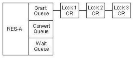
If you request a conversion of Lock 3 from CR mode to CW mode, the lock manager can grant the request because CW mode is compatible with CR mode, and there are no lock conversion requests on the convert queue. The following illustrates the state of the lock queues after this request.
